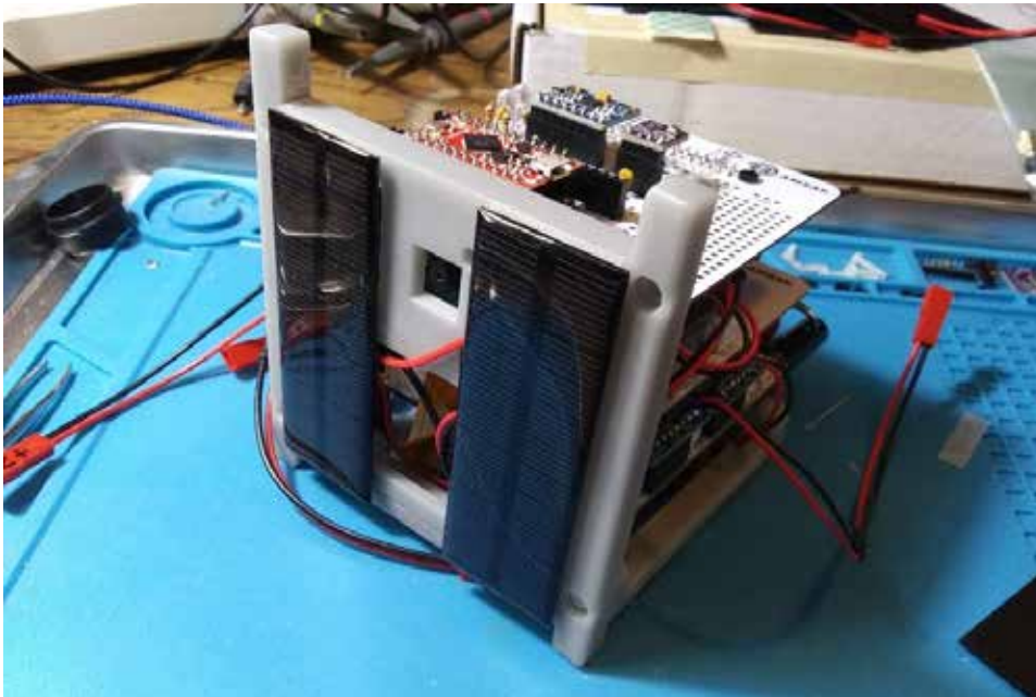
Figure 6 — +Y side of the sim with the Pi camera installed: the small solar panels had a slightly different configuration of the power contacts than the ones on the BOM, so connecting them in parallel left a wire or two showing.
