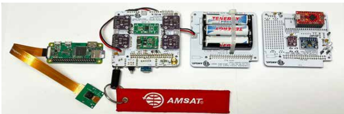
Figure 3 — Boards of the CubeSatSim. From left to right, the Pi Zero WH with Pi Camera, Mainboard, Battery board, and STEM Payload board with Sparkfun Pro Micro microcontroller.
